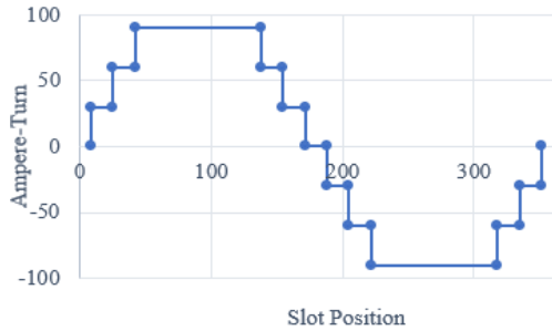
Fig. 3. Ampere-turn step distribution of reference motor (180 turns per phase per pole-pair, 90 A-turns peak value).
