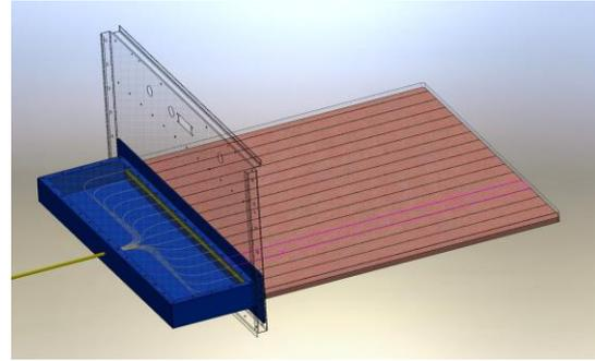
**Fig. 2.** Ingress/ egress of the FBG's and wiring bundle
