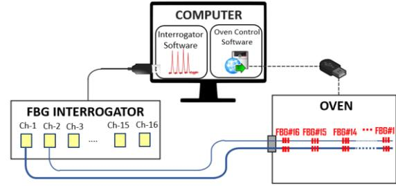
Fig. 1. Schematic representation of sensor calibration set-up
