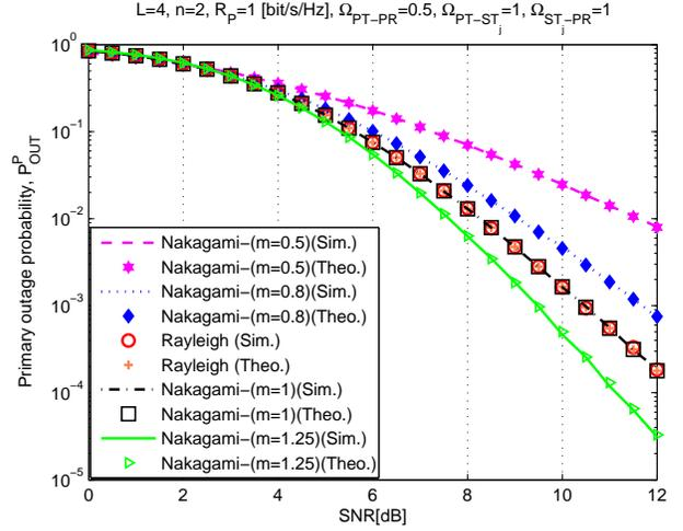
**Fig. 4:** Comparison of Nakagami- $m$  with Rayleigh fading channels. When  $m=1$ , Nakagami fading corresponds to Rayleigh fading.
