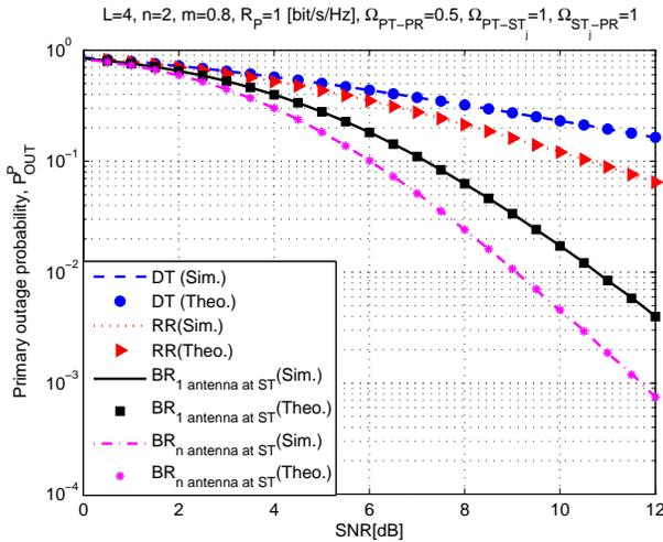
**Fig. 3:** Performance of DT, RR, BR with one and multi-antenna over Nakagami- $m$  fading channel.
