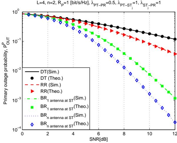
**Fig. 2:** Performance of DT, RR, BR with one and multi-antenna over Rayleigh fading channel.
