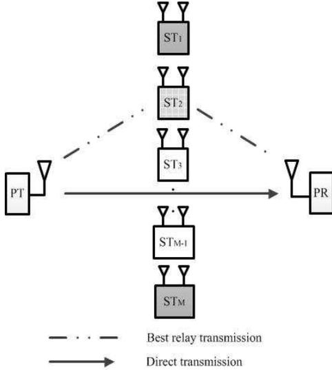
**Fig. 1:** System model under consideration. The dashed-dotted line indicates that the best relay (CH) transmits only when cooperation is required. For simplicity, SRs are not shown.
