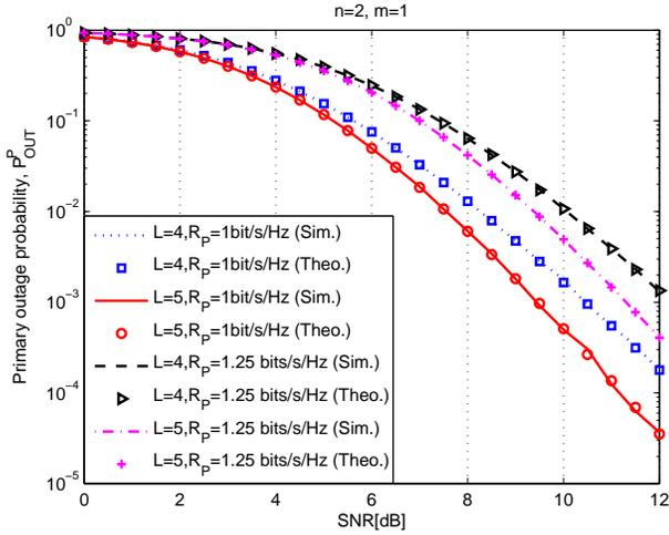
**Fig. 5:** Primary outage probability of the  $BR_n$  over Rayleigh and Nakagami- $m$  ( $m=1$ ) fading channel for varying  $L$  and  $R_p$ .
