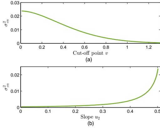
**Figure 3.** Relationships between companding noise and (a) cut-off point  $v$  and (b) slope  $u_2$
