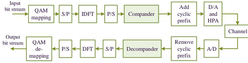
Figure 1. OFDM system model with a companding transform
