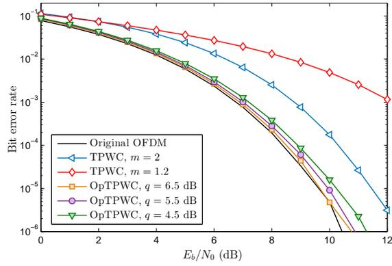
**Figure 5.** BER performance comparison of TPWC and OpTPWC over AWGN channel using 4-QAM based OFDM.  $\rho = 10^{-2}$ ,  $P = 10$  dB
