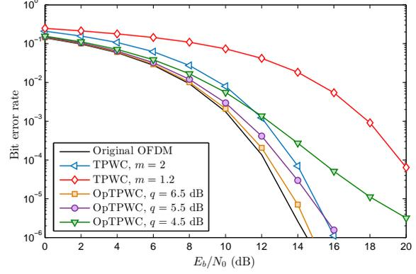
**Figure 6.** BER performance comparison of TPWC and OpTPWC over AWGN channel using 16-QAM based OFDM.  $\rho = 10^{-2}$ ,  $P = 10$  dB
