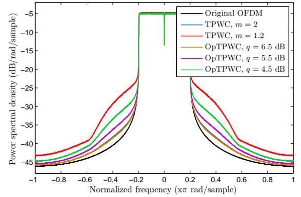
**Figure 7.** PSDs of TPWC and OpTPWC using 4-QAM based OFDM.  $\rho = 10^{-2}$ ,  $P = 10$  dB
