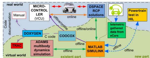
Figure 1. Framework for development a complex robotic system
