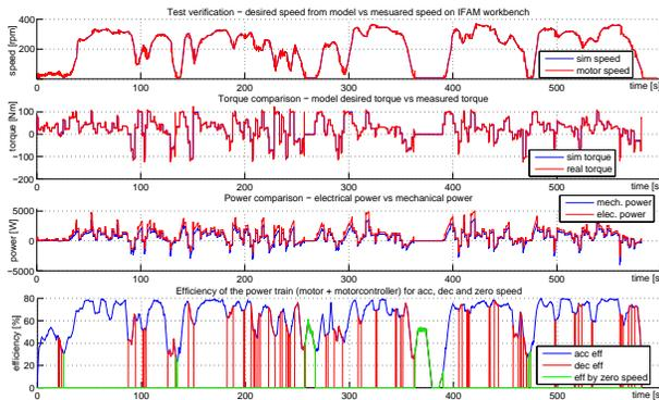
**Figure 9.** Test results of a sample trip (a724367v20) with a trip displacement of 4.16 km on EOsc2 power train with an average energy consumption of 17.9 kWh/100 km. The measured energy consumption is 610 kW and the regenerated energy from recuperative braking 59 kW.
