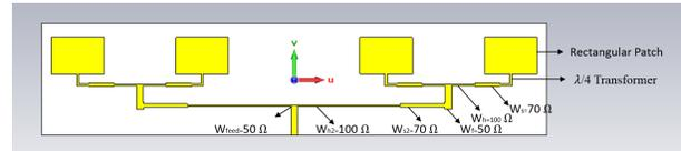
**Figure 5.** Illustration of 1x4 microstrip patch array antenna
