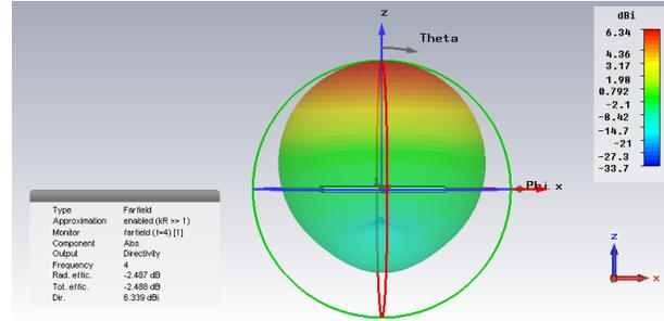
**Figure 4.** Directivity pattern of the single element antenna
