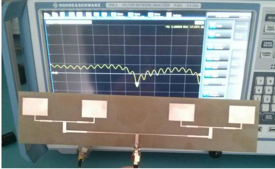
**Figure 7.** Fabricated array antenna and its  $S_{11}$  measurement
