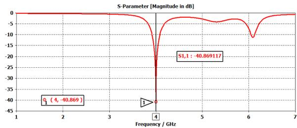
**Figure 3.** Return loss of the single element antenna
