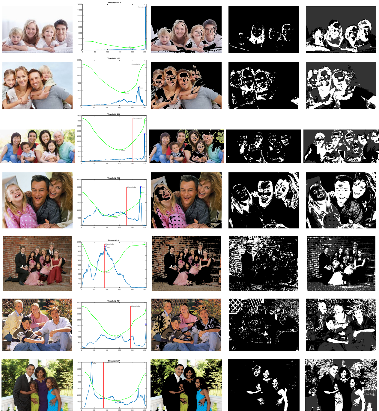
Fig. 4. Detection capabilities of our method with multiple humans on an image and complex background: (1) original images, (2) histogram with threshold, (3) image with removed background pixels, (4) detected skin pixels and (5) clustered skin color detection.
