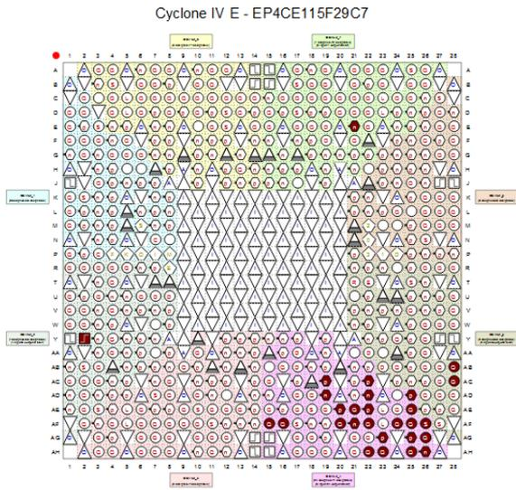
**Fig. 5.** Altera DE2-115 Pin Structure
