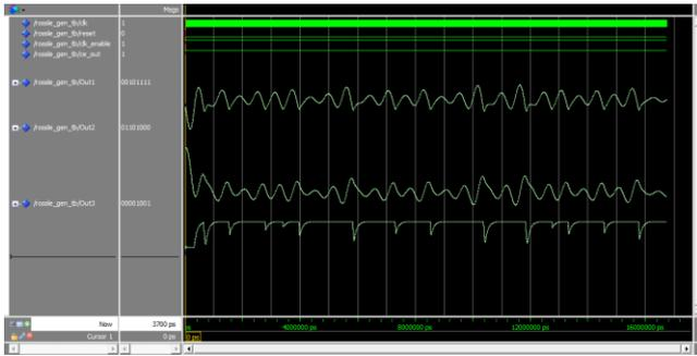
**Fig. 8.** The dynamics of  $x_1$ ,  $x_2$  and  $x_3$  with *Multisim Program*
