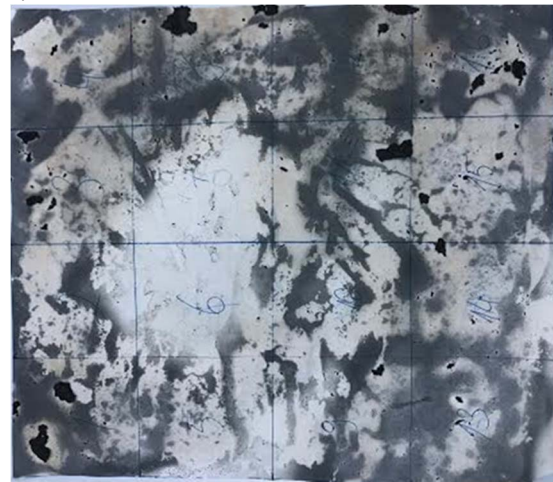
Fig. 3. Thermal fax paper stain of sample 1 during microwave drying
