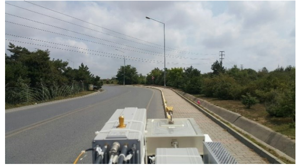
Fig. 7. Millimeter wave measurement system with power amplifier and 24 dBi antenna.
