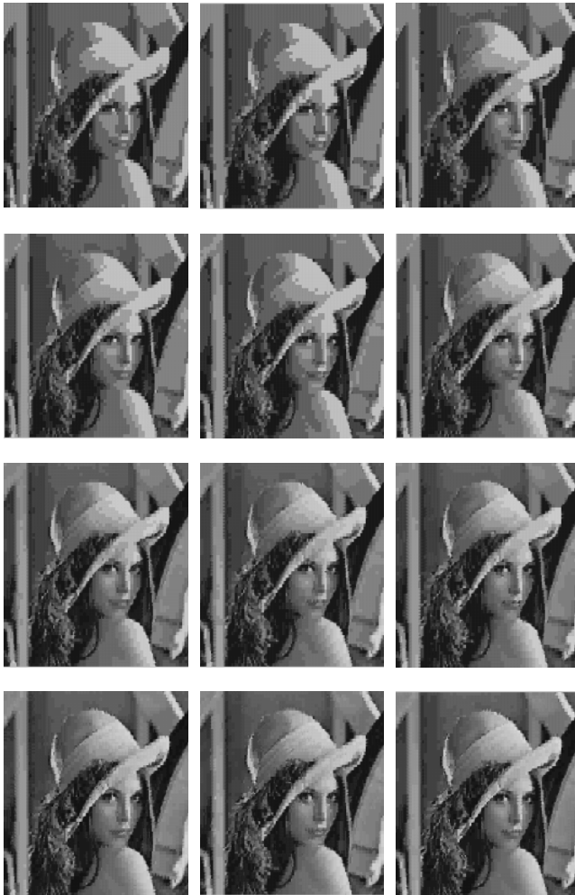
Fig. 6. Reconstruction of Lena after the implementation of GA with various natural selection in population that has 8, 16, 32, 64 codeword number from above to below row (Roulette Wheel, Elitist, Pool Based Natural Selection respectively)
