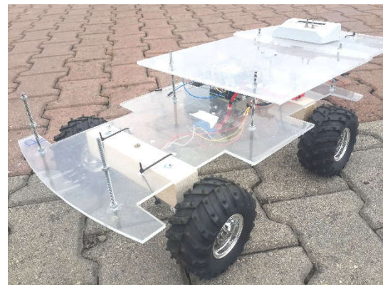
Fig. 2. Main chassis realization of GÜVE. Control panel (far top) and wheels are visible.
