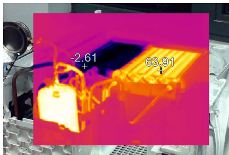
Fig. 11. Thermal image of condenser and evaporator surfaces
