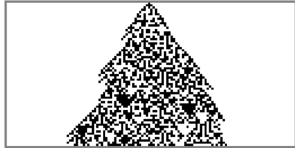
Figure 4. Evolution of the ECARMM composed of 128 cells with parameter p_m = 0.3 , m = 0, 1, \dots, 127 and Rule 150 for 64 time steps.
