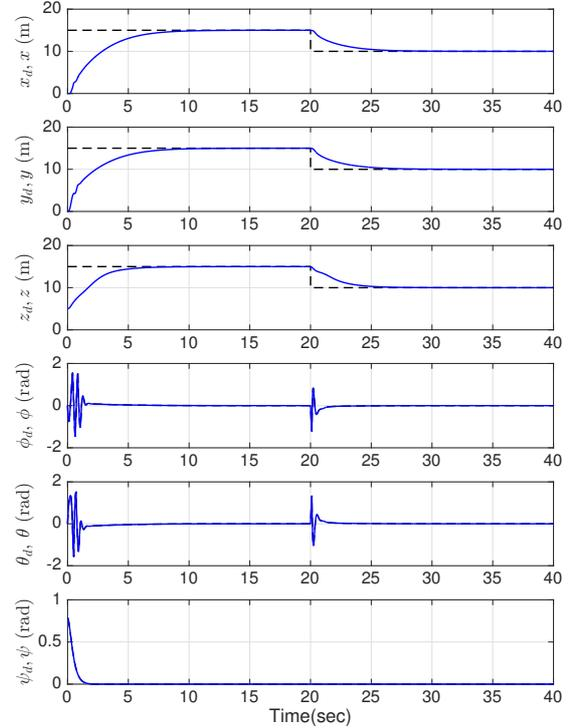
**Figure 1.** Results for simulation #1: Change of position and attitude signals (Reference signals are given in dashed (black)).
