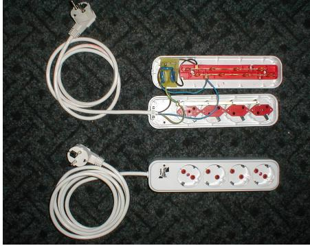
**Fig. 3. 'Multi-plug Block Protected from Overvoltage – BMS-01'**
