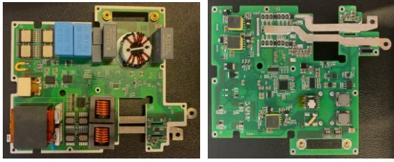
Fig. 8. Top view at left and bottom view at right of implemented PSFB with CDR converter
